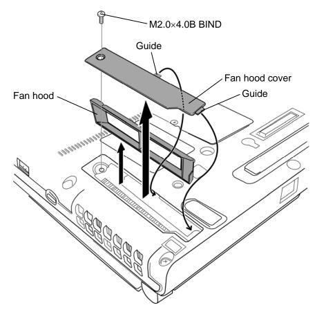
Figure 4-13 Removing the fan hood
